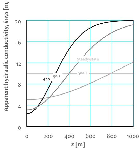
Figure 4. Apparent hydraulic conductivity in the confined aquifer.
