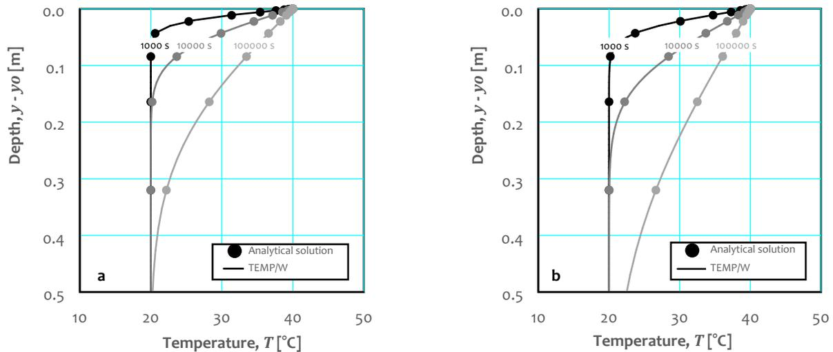
Figure 2. Temperature profile. (a) Conductive heat transfer. (b) Conductive and radiative heat transfers.
